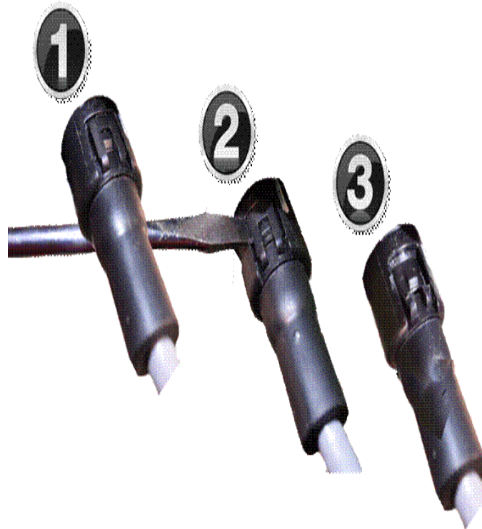
Figure 3. Locate locking tab (1), lift up on the tab with a screwdriver (2), snap tab off (3).
