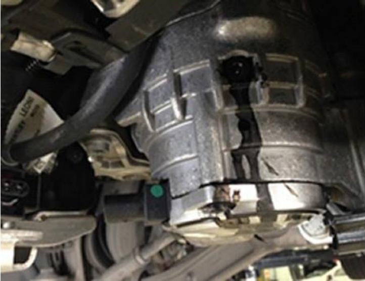
Figure 1 Active engine mount leaking oil
