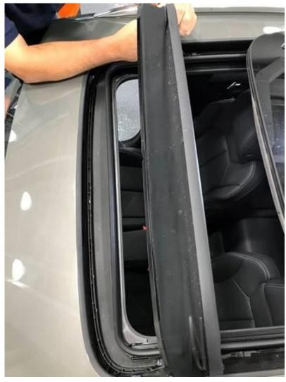
Figure 2. Front sunroof opening with drainage exposed.
