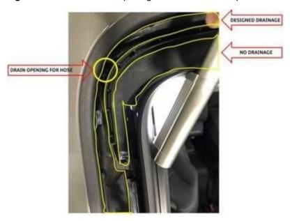
Figure 4. Sunroof water channeling diagram.
