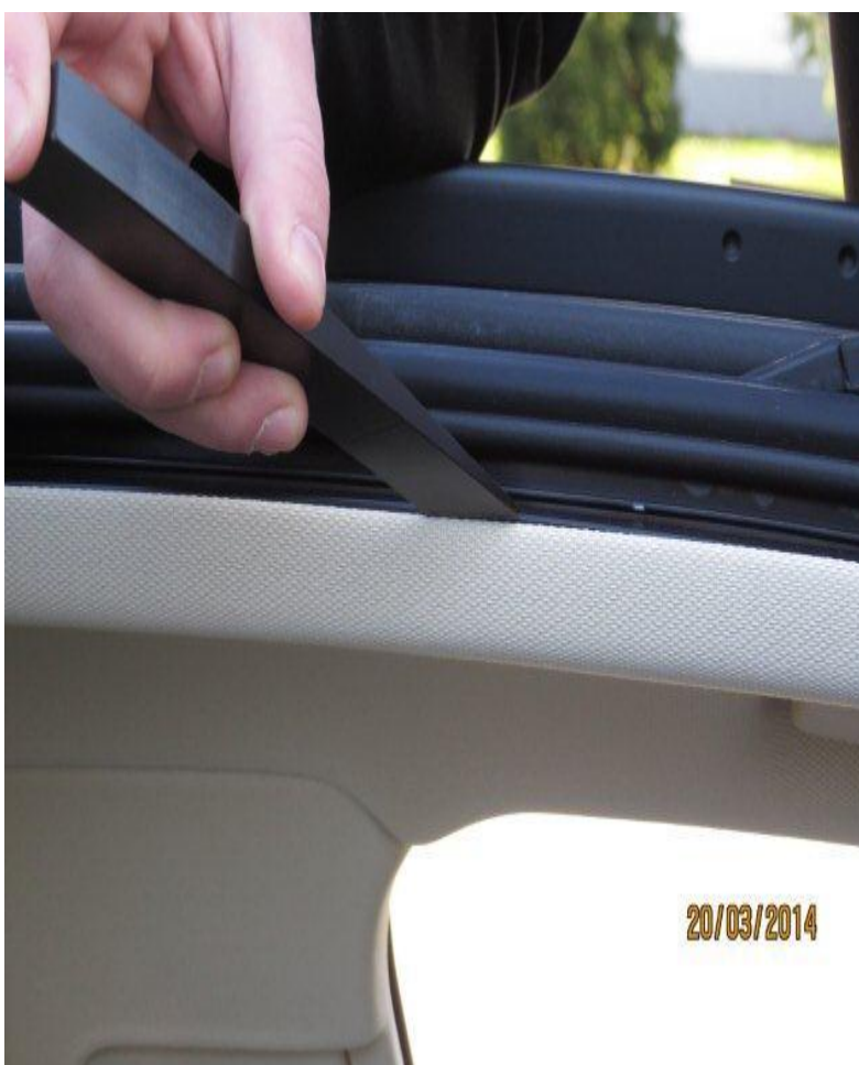
Figure 1. Unclipping the sunroof cover trim frame.
