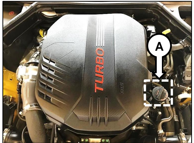
Stinger (CK) 3.3T engine is shown above for demonstration purposes only. Location of engine oil filler cap may vary on different models.
