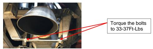
Slide the lower upper exhaust pipe in the lower proheat exhaust pipe and secure them with the existing clamp, U bolt, and nuts.
