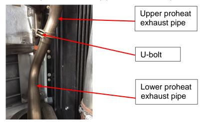
Remove and save the nut securing the lower proheat exhaust pipe to the bracket on the coach. Slide-out the lower proheat exhaust pipe and save it.
