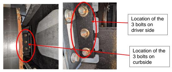
Secure the bumper to the coach frame in the engine access door compartment using the existing bolts removed in Step2 and torque them to 18-22 Ft-Lbs.
