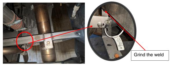
Install the new LH skid plate bracket, MCI P/N: T03-3077, using the hardware removed in the previous step.
