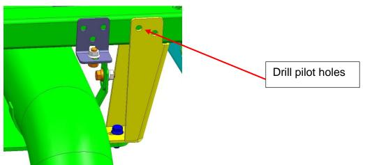
Match drill the holes in the bracket using a 25/64 drill bit.
