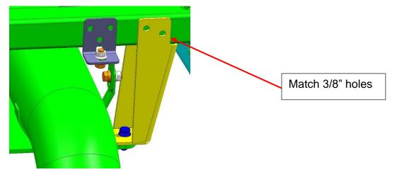
Using the 3/8-16 bolt (MCI P/N: T19-1170, 3/8-16 nut (MCI P/N: T19-1171), 3/8 washer (MCI P/N: 19-2-63), and 3/8 lock washer (MCI P/N: T19-1172) secure the RH skid plate bracket to the coach frame. Torque the bolts to 20 Ft-Lbs.
