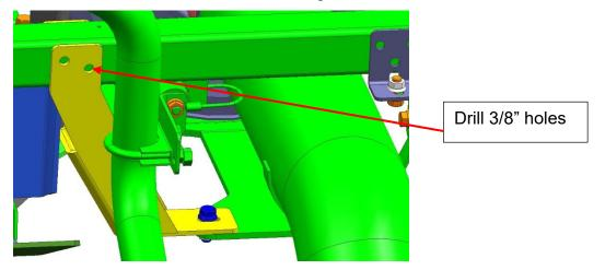
Using the 3/8-16 bolt (MCI P/N: T19-1170, 3/8-16 nut (MCI P/N: T19-1171), 3/8 washer (MCI P/N: 19-2-63), and 3/8 lock washer (MCI P/N: T19-1172) secure the LH skid plate bracket to the coach frame. Torque the bolts to 20 Ft-Lbs.
