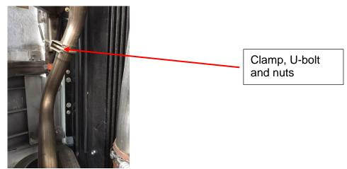
Secure the lower proheat exhaust pipe to the bracket on the coach using the existing nut.
