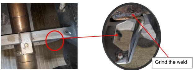
Install the new RH skid plate bracket, MCI P/N: T03-3076, using the hardware removed in the previous step.
