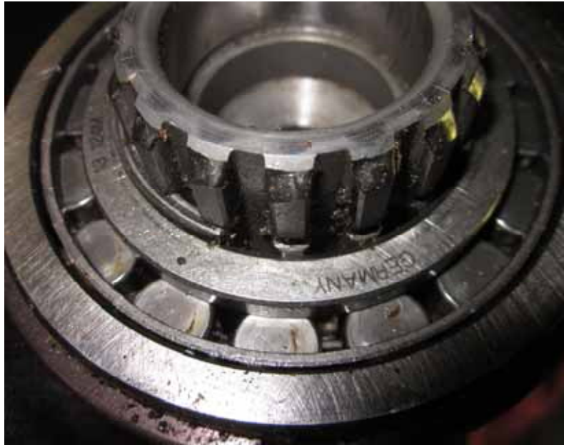
Pieces of ring get into the PTO and cause operational issues.
