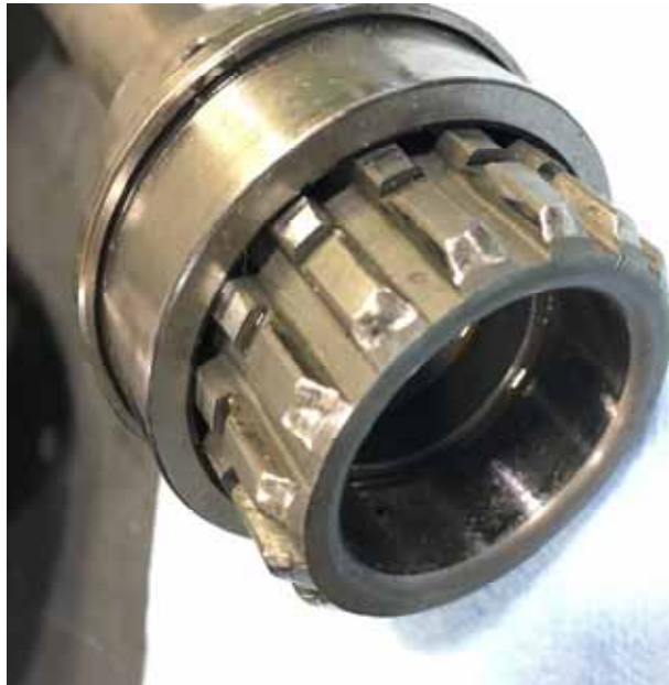
Pieces of ring get into the PTO and cause operational issues.
