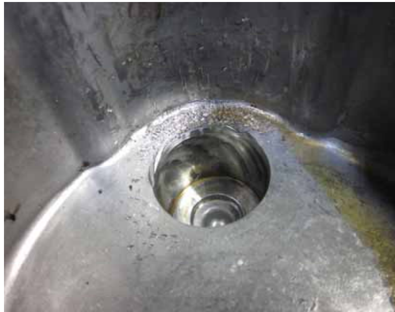
PTO case damage from snap ring or other debris can be cleaned up and inspected. If the damage does not affect the operation of the PTO shifter and piston seals the PTO can be repaired.
