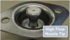
NOTE: The high flow and the low flow aftertreatment hydrocarbon dosers have different flow rates.
