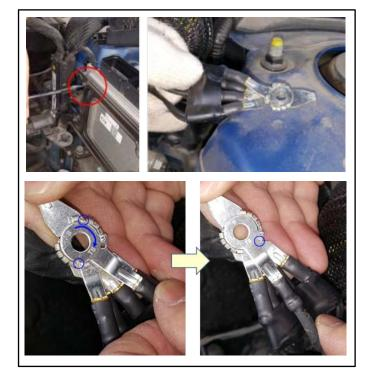
12. Cut off and discard the original terminals from the ECM connector and fold the original wires (K) back onto the original engine control wire harness and secure with tape. Secure any excess wire from the new wire harness extension onto the original engine control wire harness with tape.
