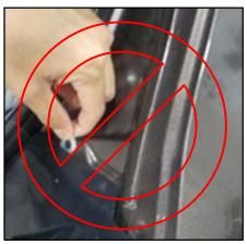
This is to prevent the washer from falling into the gap between the body and the lamps.
