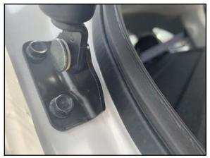
6. Confirm that the washer is completely inserted and that the popping noise is gone when opening and closing the tailgate.
