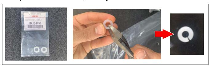
4. Using your hands, spread the washer open at the slit, as shown.
