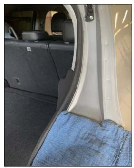
2. Before starting, keep tailgate in the open position and cover the gap above both rear combination lamps (LH and RH) with a cloth.
