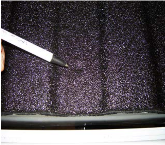
Spot weld under bed liner example
