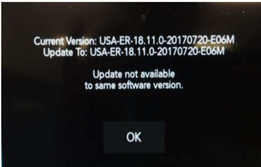
Fig. 5 Screen Displayed When Radio Software Level Is Up To Date (figure is for reference only)
