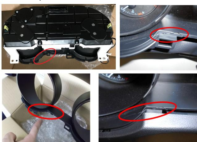
Use the photos below for reference when **CAREFULLY** removing the combination meter lower trim bezel.
