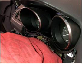
**Step 10:** Plug the AC adapter of the reprogramming tool into 120v AC "house current" and the combination meter harness connector into the meter. The meter will power up and illuminate completely. The tool's Yellow LED will illuminate. Press the black button to start the update. It takes about 70 seconds to complete.
