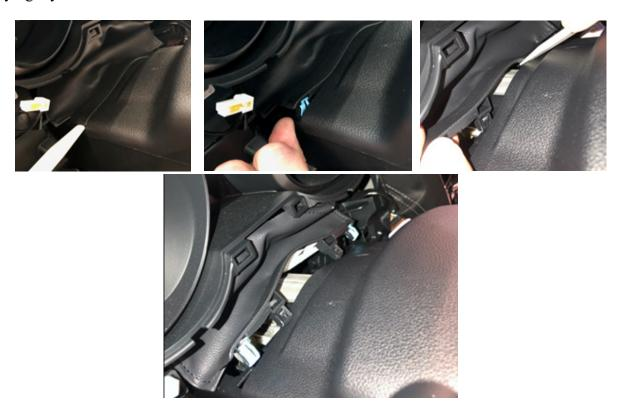
**Step 8:** Remove the 2-10mm bolts from the underside of the visor and the 2 philipps screws on the bottom corners of the combination meter. **TIP:** Use a finger under the head of the screw to keep from dropping it inside the IP.
