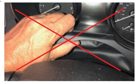
Reports of damaged meter housings as shown in the example photos below have necessitated revisions to this step.
