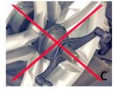
**Figure 3**. Five-finger style clamping plate (A), wheel properly mounted with a five-finger style clamp (B), and wheel mounted using an incorrect clamping tool/method (C).
