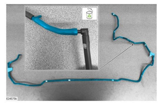
Remove and discard the section of active engine mount vacuum hose.
