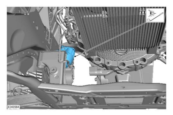
Inspect the active engine mounts for signs of excessive wear and/or leaking fluid.
