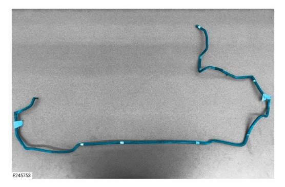
The illustration shows the active engine mount vacuum hose removed from the vehicle.
