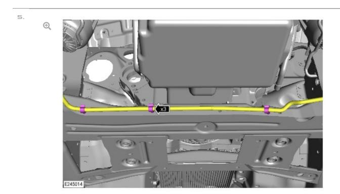
Disconnect the active engine mount vacuum hose from the fasteners.
