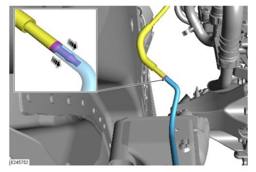
Separate the active engine mount vacuum hose at the connector shown in the illustration.
