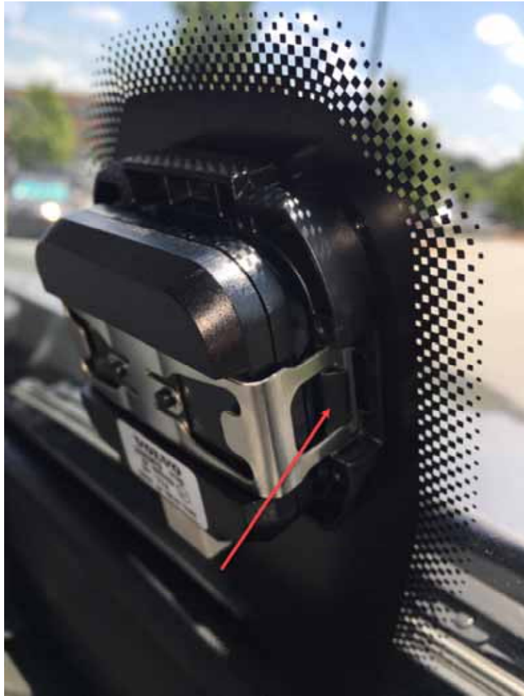
2a. Removed sensor, position sensor and wire out of the way for damaged windshield removal
