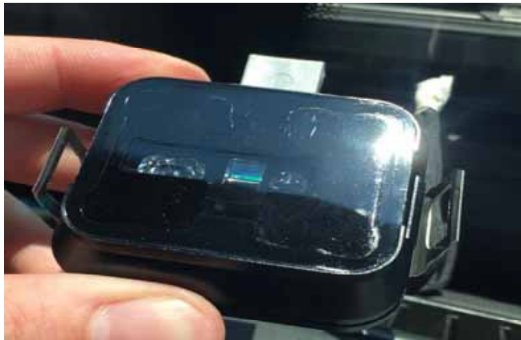
3. Begin by using the heatgun to heat the adhesive on the current bracket.
