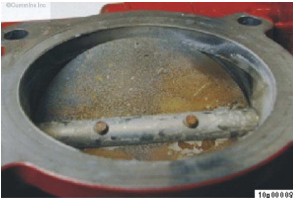
Figure 8, Throttle plate with flux deposits
