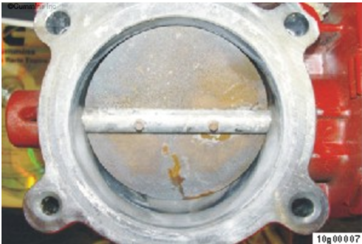
Figure 6, External deposits seeping from ISL G CM2180 fuel module near the wastegate control valve
