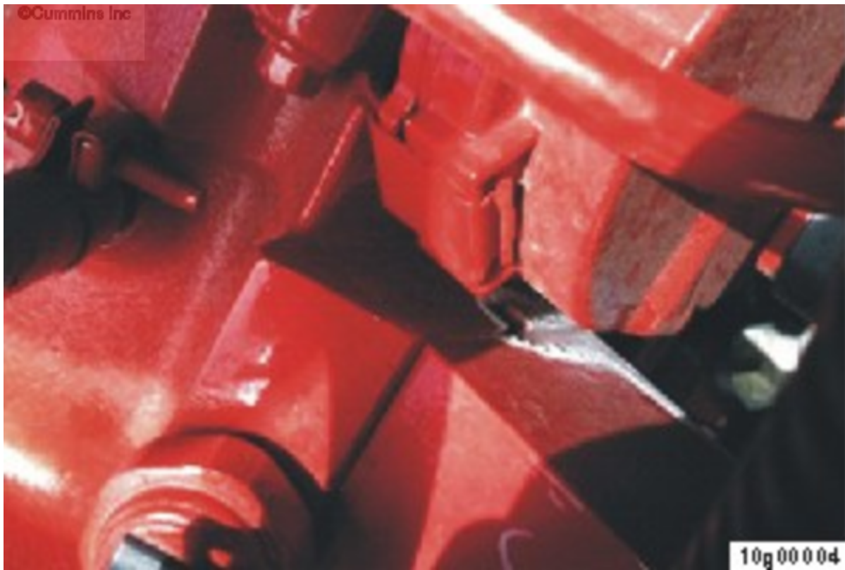
Figure 6, External deposits seeping from ISL G CM2180 fuel module near the wastegate control valve
