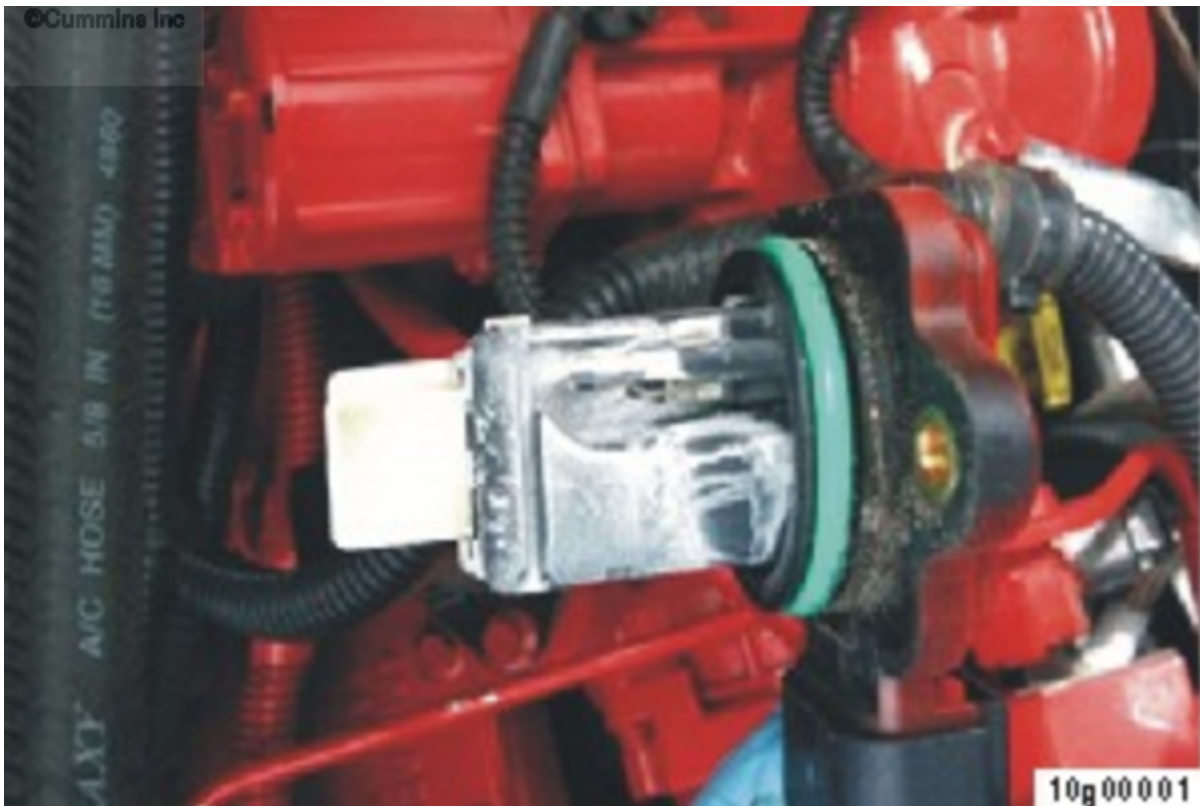
Figure 4, Air/fuel mixer with flux deposits
