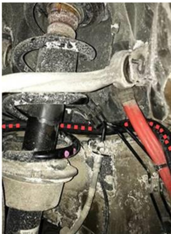
Figure 6. Routing the rubber hose.
