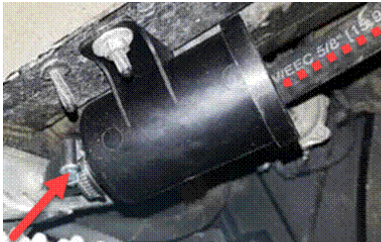
Figure 4. Connecting the NLVD filter.
