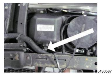
1. Locate the fuel tank filler hose to fuel tank connection.
