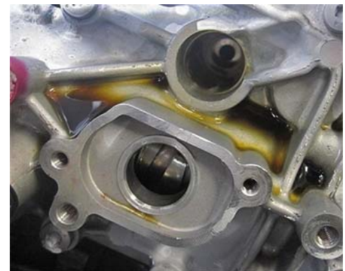
Fault type 2: Cylinder head cover leaking
