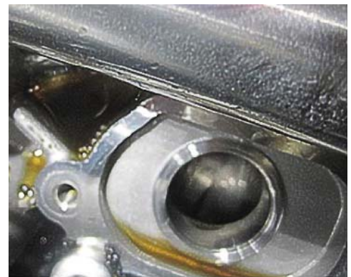
Fault type 1: Valve lift adjustment solenoid hydraulic valve leaking
