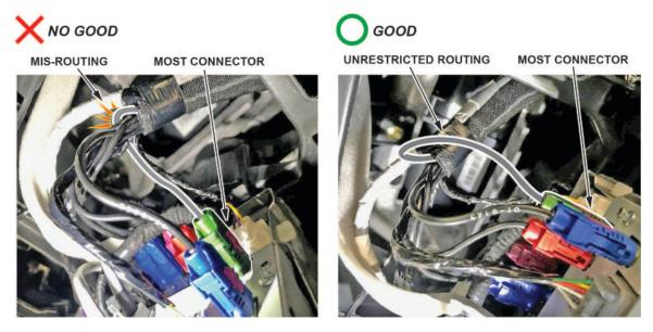
We've also found that the MOST connectors on the DVD player may get pinched between the unit and the air ducting box. We don't have a permanent fix for this, but you can try adjusting the wires to take pressure off of them.
