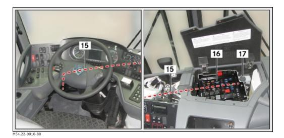
10. Route electrical line (15) correctly along the existing wiring harness to the position of old diagnostics connector (17) and secure it using cable ties.
