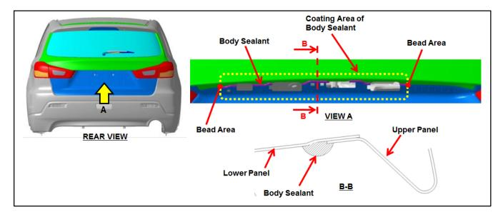
3. Using a spatula, wipe off excess sealant on the edge of the upper panel and surface of the lower panel. Wipe off any sealant on the edge of the hole for the liftgate open switch.
