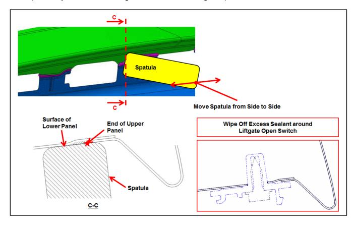
**NOTE:** Ensure there is sufficient sealant between the upper and lower panels, and the sealant surfaces are smoothed out flush with the body panel surfaces.
