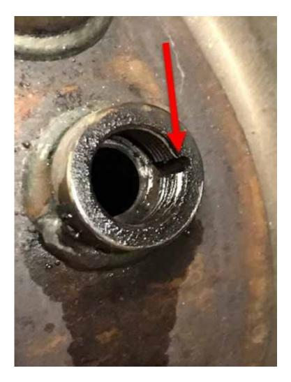
**6.** Install the new PM sensor and torque to spec. Refer to <u>Impact</u> for the correct torque spec.
