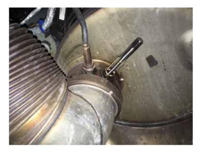
**5.** Inspect the boss threads and PM Sensor alignment notch for debris and clean if necessary.
