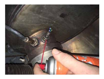
**3.** Remove the sensor with a  $\frac{1}{2}$ " drive impact and appropriately sized deep socket.
