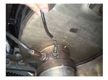
**2.** Spray the sensor nut with a suitable rust penetrant and let soak for approximately 5 minutes.
