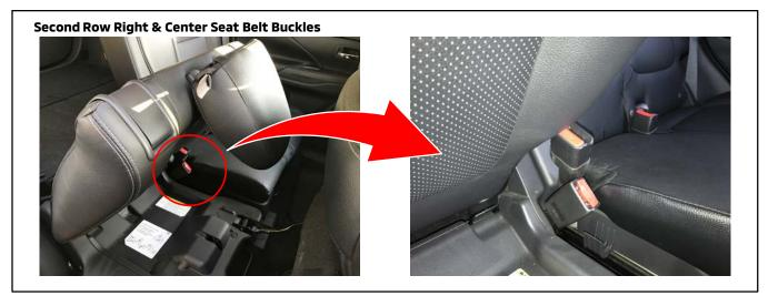
The second row center seat belt buckle length has been shortened by 14 mm to prevent the center seat belt buckle from covering the right side seat belt buckle.
