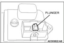
Once the tab is disengaged, lift the door lock switch off the switch. Ensure the plunger is free from foreign material or debris.
