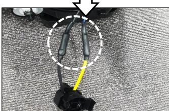
11. Insert the removed headlamp bulb back into the new connector.
