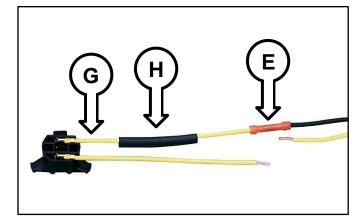
8. Crimp the new connector wire end to the head lamp butt connector as shown. Repeat steps 7 and 8 for the other wire.
