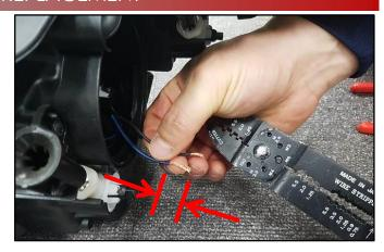
Insert the stripped headlamp wire end (F) into the butt connector (E). Crimp the connector to the headlamp wire. Repeat for the other wire.
