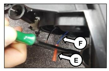
7. Insert the new connector wire (G) through the shrink sleeve (H) before inserting the connector wire end into the headlamp butt connector (E).
