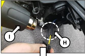
10. The completed repaired wires with new butt connector should look as shown.
