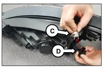
Using a set of wire cutters, cut the two
