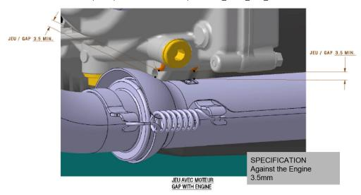
Note the Exhaust too close will reveal marks on the frame and exhaust pipe. If no marks, the problem is possibly somewhere else.
