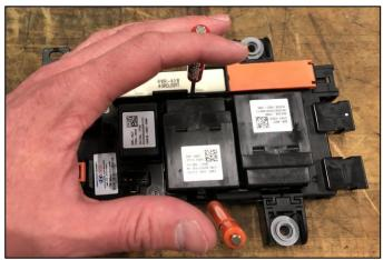
5. With the screwdrivers inserted remove the main relays with Oil Filter Pliers, Water Pump Pliers, or a similar tool.
