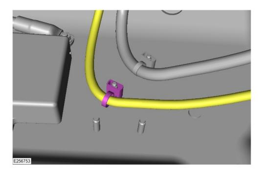
Install the new retaining clip and secure to the vehicle startup battery positive (+) cable to the loadspace floor stud as shown.
