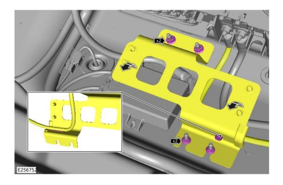
Position the RDCM mounting bracket to allow access to the vehicle startup battery positive (+) cable.
