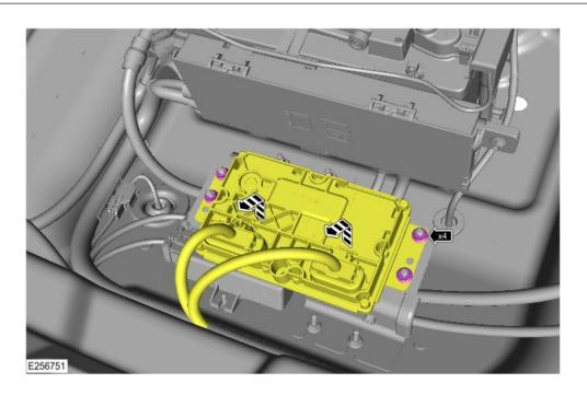
Position the Rear Differential Control Module (RDCM) to the side.
