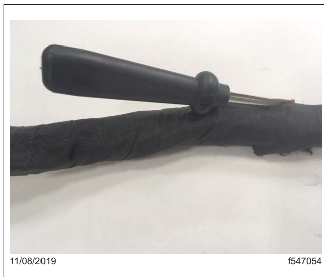
Fig. 9, Cutting an Opening into the Fiber Wrap
