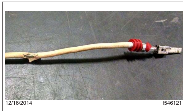
Fig. 2, Insulation Discoloration, Major
