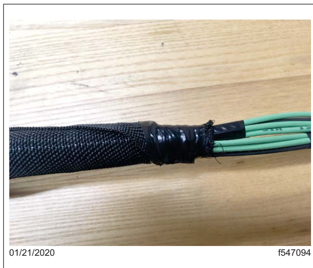
Fig. 7, Harness Wrapped with TwistTube®
