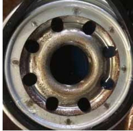
Corrosion/rust on secondary filter
