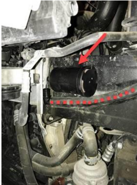
Figure 3. Installing the new NLVD filter.
