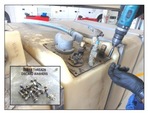
2. Remove the two tank fillers from the old tank; clean flanges and threads (discard old gaskets).
