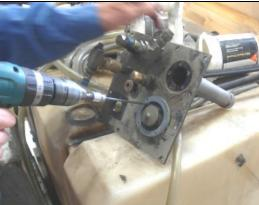
7. Secure the plate in a vice and reinstall the top and bottom hose fittings on the new accessory plate using thread sealant on the fitting threads (do not install fuel sender or valves).
