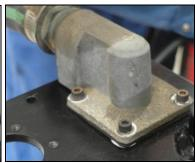
9. Install the two part pressure valve with lower gasket # 531427 (put sealant on the threads) and upper gasket # 531428.
