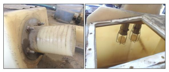
3. Reinstall the filler tubes on the new fuel tank using the two supplied gaskets # 032938. Reuse the filler tubes hardware and apply Teflon paste on the stud threads.
