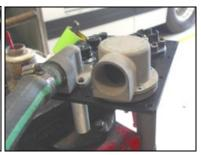
10. Install the fuel sender and cork gasket # 531419 (put sealer on the hex screw threads).
