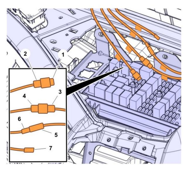
Install new fuses into the FRC (Fuse and Relay Centre).
