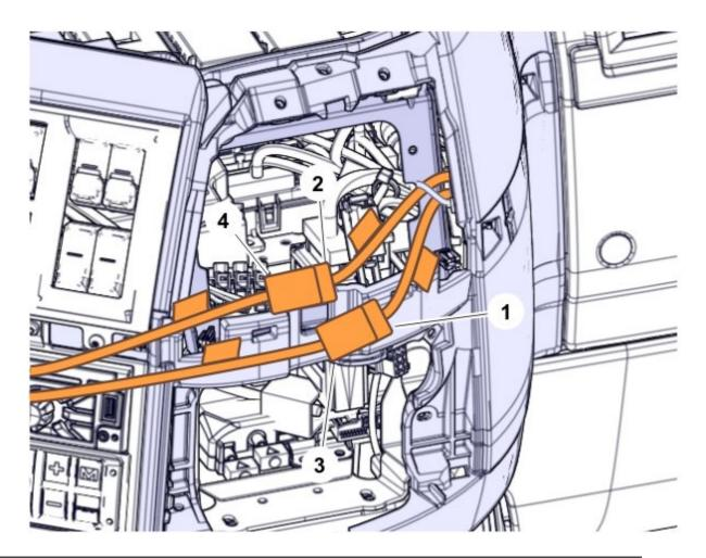
Transfer the terminating resistor to the overlay cable harness.
