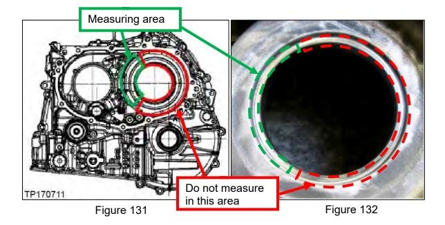
$\mathbf{Y}$  = The distance between the upper surface of the Gauge Block J-50271 and the surface where the snap ring seats.
