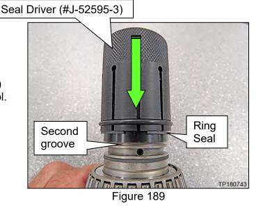
• Confirm that both of the Ring Seals are not protruding in any direction.
