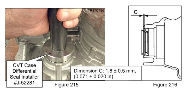
194. Install the differential side oil seal to the converter housing (Figure 217).
