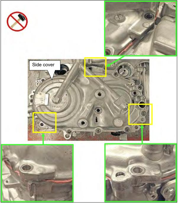
78. Align the primary pulley bearing retainer bolt holes with the bolt hole on the case as shown in Figure 98.
