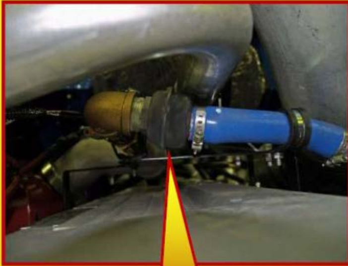
DPF Combustion Air Check Valve
