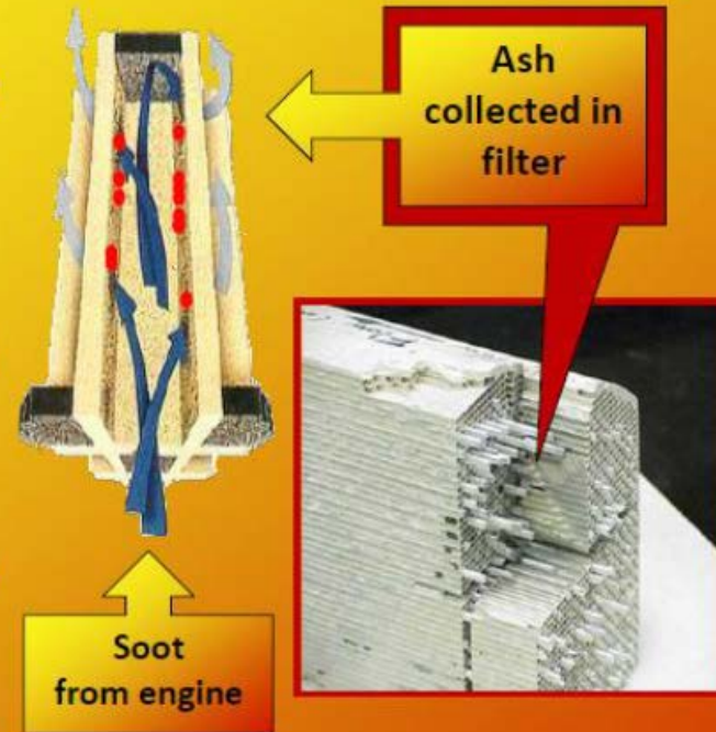
Cordierite (Ceramic) Honeycomb Filter Substrate
