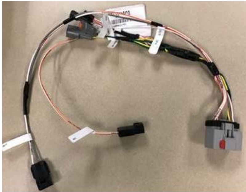
23295906 = From the RP1226 to a 9 pin connector.
