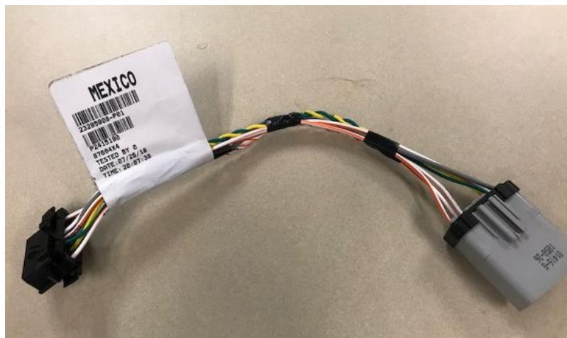
23295908 = From the RP1226 to a 16 pin connector.
