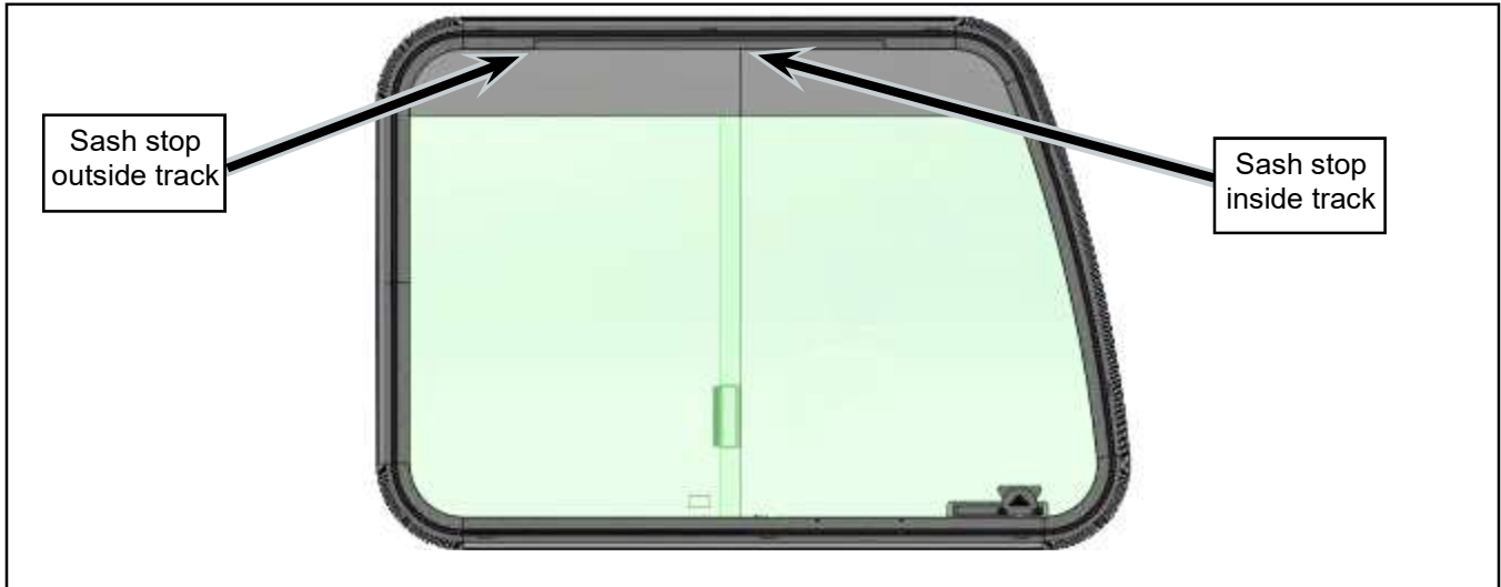
Figure 2 - Sash Stops Location
