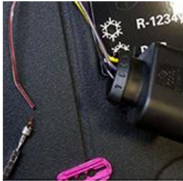
Figure 1. T4e with damaged wire.
