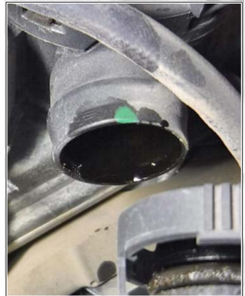
Vent line on oil separator
