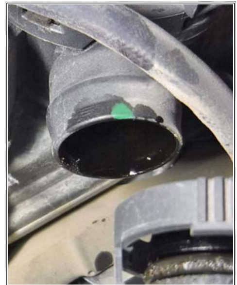
Vent line on oil separator
