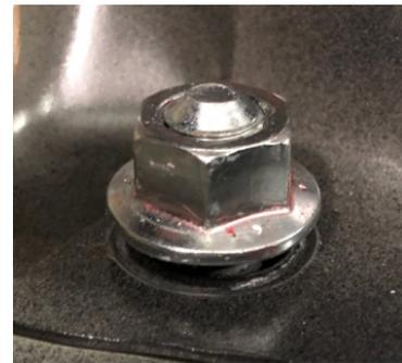
**Step 5)** Remove both front (closest to the rear seat backrest) retaining nuts and discard them as they are **one-time use** items. Loosen (but do not remove) the rear nuts. Loosen them enough so the top of the nut aligns with the taper at the start of the threads as shown above. This will allow movement of the shock absorber assemblies making it easier to remove from the lateral links and keeps them from dropping out of the vehicle after removal.
