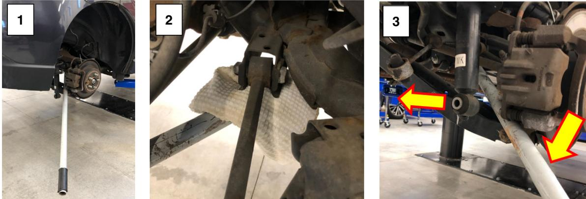
**Step 8)** Remove and discard the other top retaining nut loosened in **Step 5** and remove the affected shock absorber assembly from the vehicle.
