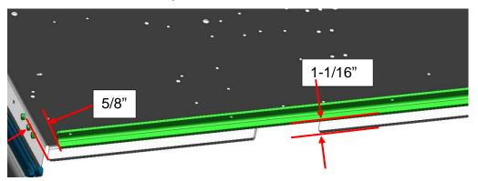
Install angular support using screws, MCI P/N: 19-1-630, nuts, MCI P/N:19-3-11, and washers, MCI P/N:19-2-102.
