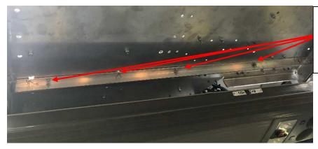
Install the support using screws, P/N: 19-1-630, nuts, P/N:19-3-11, and washers, P/N:19-2-102
