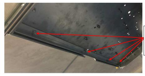
Install the support using screws, P/N: 19-1-630, nuts, P/N:19-3-11, and washers, P/N:19-2-102
