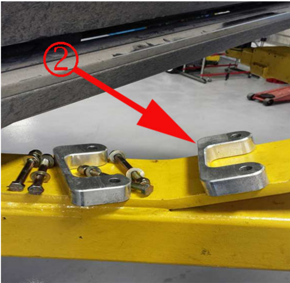
2. Aftermarket lift kit blocks removed from a truck
