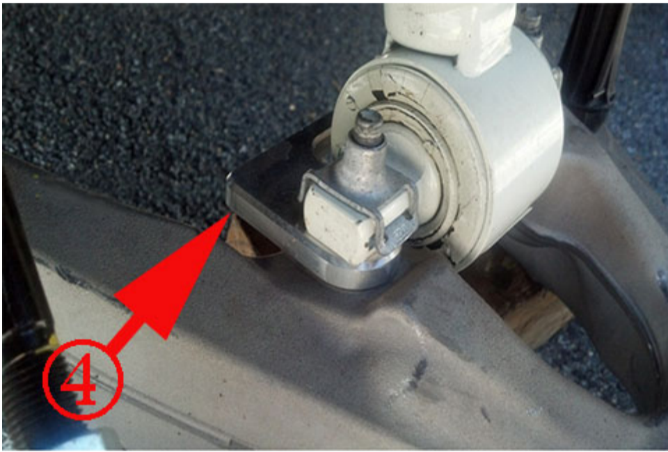
4. Aftermarket lift kit blocks installed
