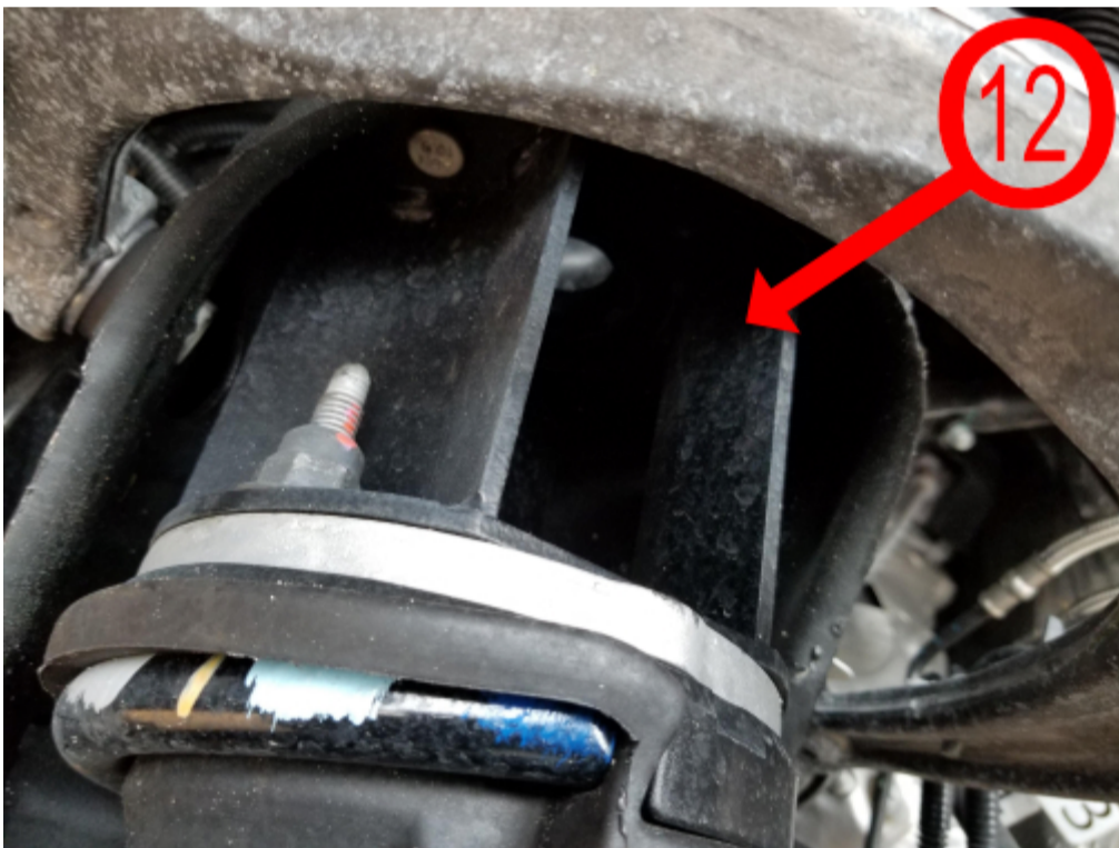
12. Aftermarket Coil Spring Spacer installed
