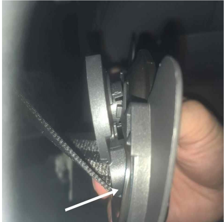
Figure 5. Installing modified seat belt guide starting with the metal tab on the bottom.
