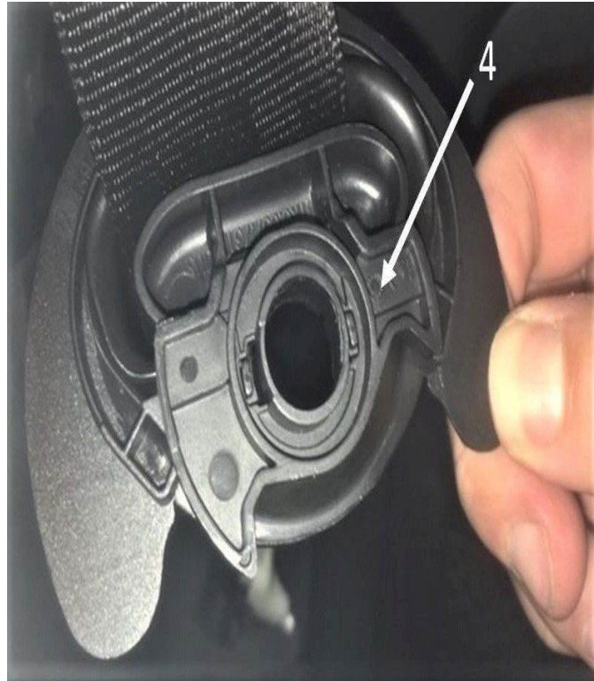
Figure 2. Backside of seat belt deflector. Deflector trim tabs engaged in old belt guide.
