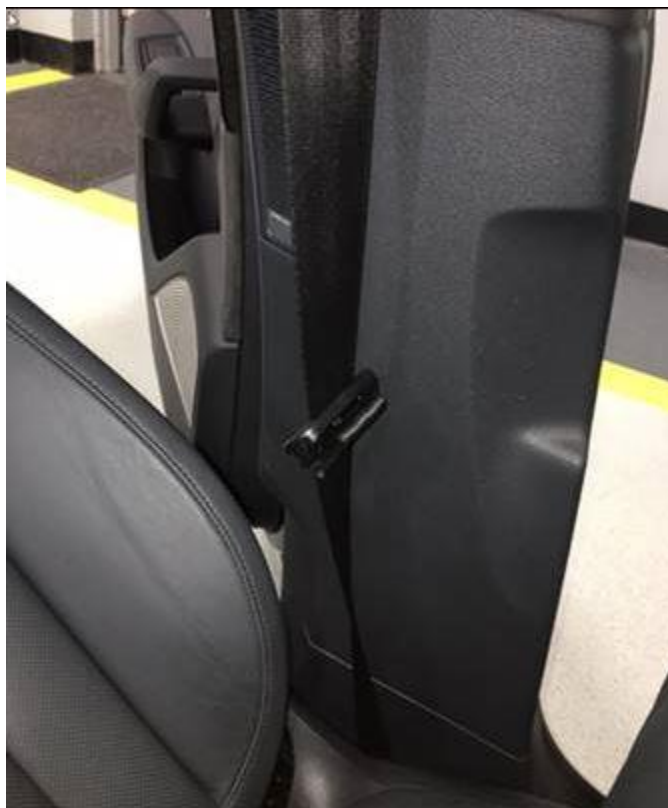
Figure 10. Example of a twisted seat belt.
