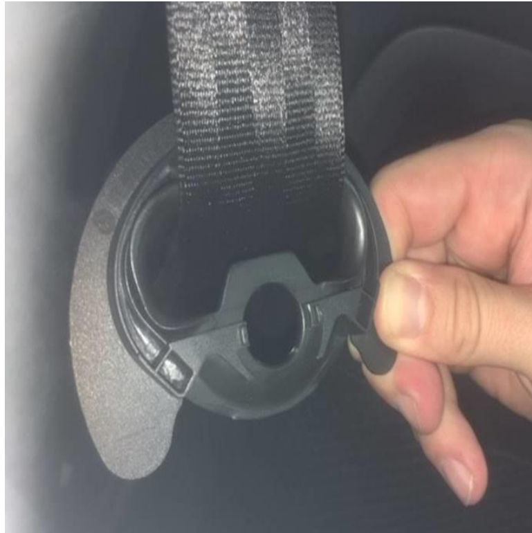
Figure 4. Old seat belt guide removed. Seat belt twist corrected.
