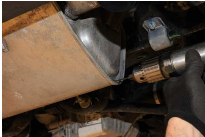
Fig. 1 Muffler Assembly With Weep Hole
