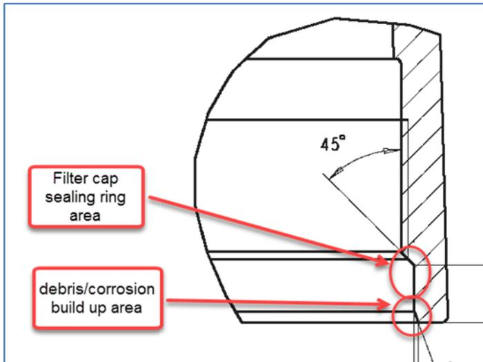
Inspection and cleaning of the sealing surface for the cap o-ring is important to avoid this damage. When cleaning is required DO NOT use power tools or grinders to clean the sealing area as this can damage the housing beyond repair. Gently scrape by hand or use abrasive paper to clean the area. If the area cannot be reliably cleaned or there is damage to the sealing surface for the o-ring, the housing must be replaced.
