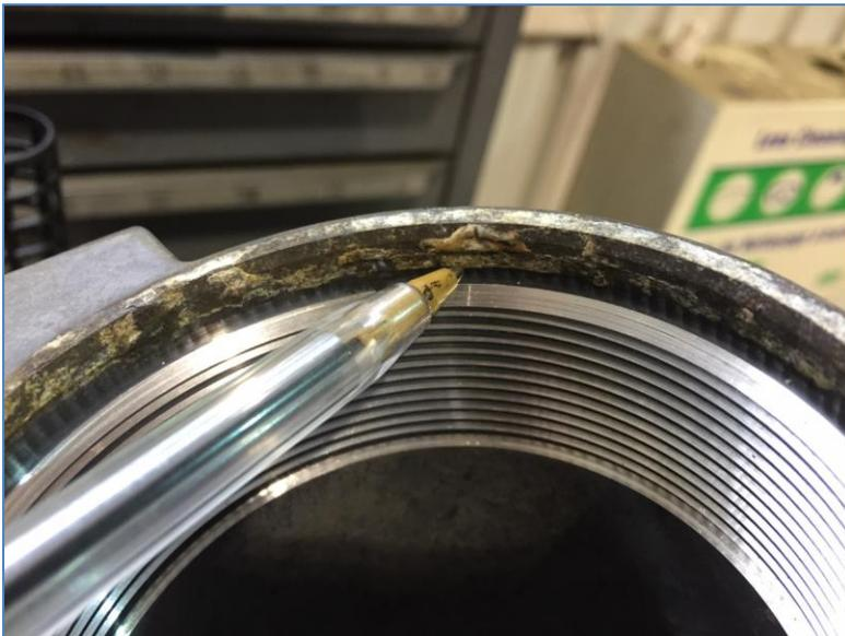
If you detect corrosion on the location shown above do not attempt to clean or reuse this housing. The corrosion is harder than the aluminum. This housing must be replaced.
