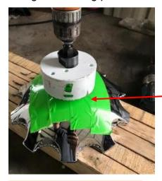
Apply masking tape and drill a 3" hole in the new hub cover, P/N: 15-01-1163
