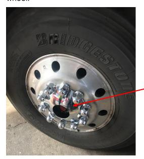
Install the modified hub cover using nut caps
