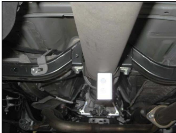
Figure 11. CORRECT Placement of Digital Angle Gauge
