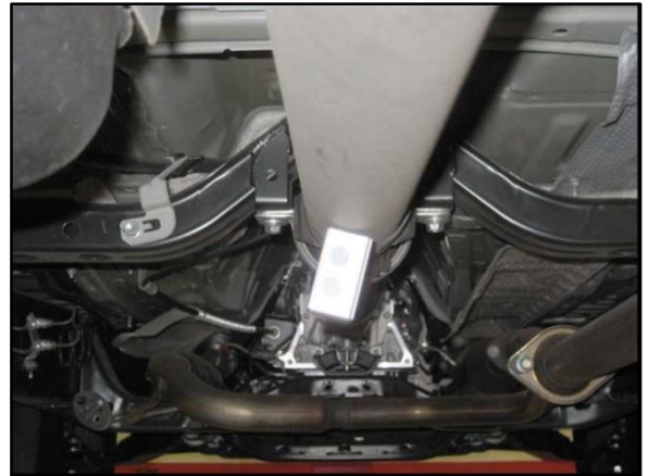
Figure 12. INCORRECT Placement of Digital Angle Gauge
