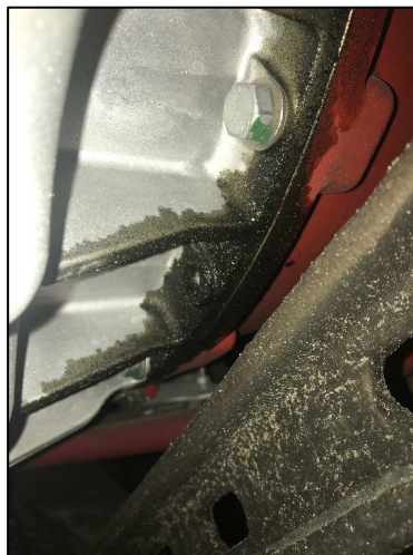
Figure 1: Traces of lubricant at the bottom of the transmission bell housing
